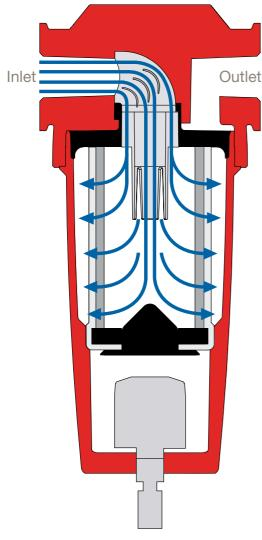
Providing an optimal flow path for the compressed air through Outlet the filter housing and element is key to reducing system operating costs
