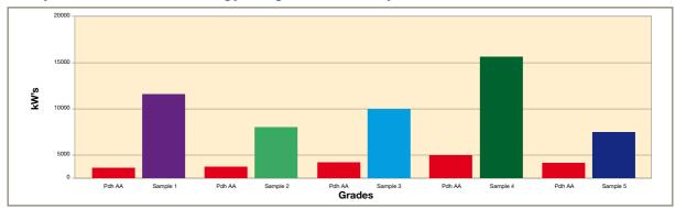
This calculation based upon a 75kW compressor operating for 4000 hours
