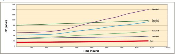
Test criteria: Filters were tested at their full rated flow and injected with ISO 12103 A4 course test dust using a pressurised dust injection system. The dust was injected in 12 intervals to simulate the monthly loading of the filter element and show a total annual differential pressure curve. OIL-X EVOLUTION filters were tested at an identical flow rate to the comparative filter and with an identical dirt loading.
