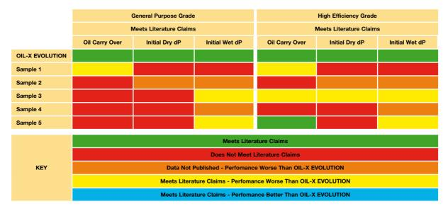
Filters tested Pdh General Purpose & High efficiency Grades against nearest equivalents. Test method used: ISO12500-1. Results independently verified by Lloyds Register.
